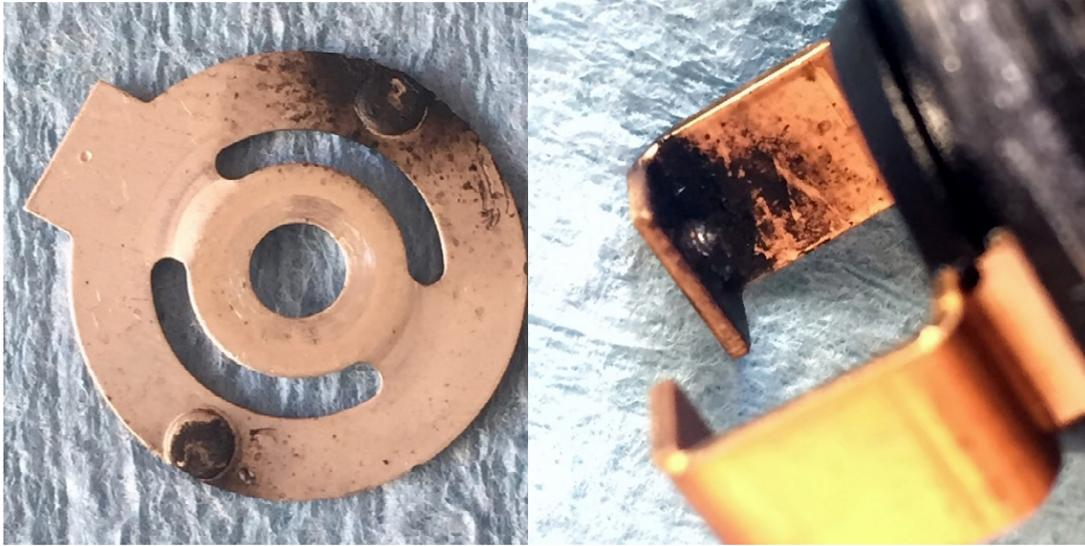
Figure 1: Arcing damage to a Lancair pressure switch due to inductive loads
